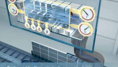
» EcoSmart AC – The control software optimally regulates the air supply units and air recirculation units
