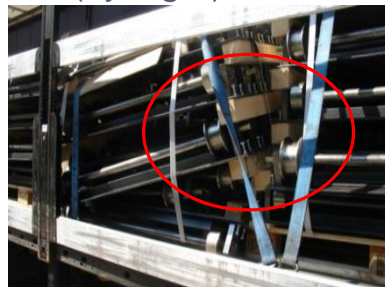
Wrong tie down, Belt no placed properly
