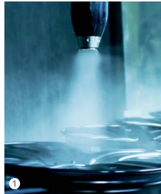
Figure 1: MAPSA's new painting line will feature a complete automatic liquid paint application system with electrostatic EcoBell 2.
